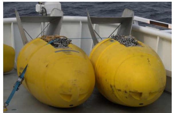
Figure 6. Two dilt floats on deck (upside down) showing the twin-fin subsurface structure
