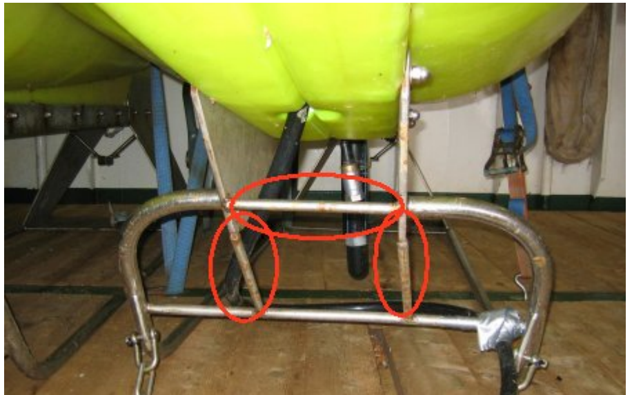
Figure 9. Simple exclusion 'turtle guard' design (the added structures are circled in red)
