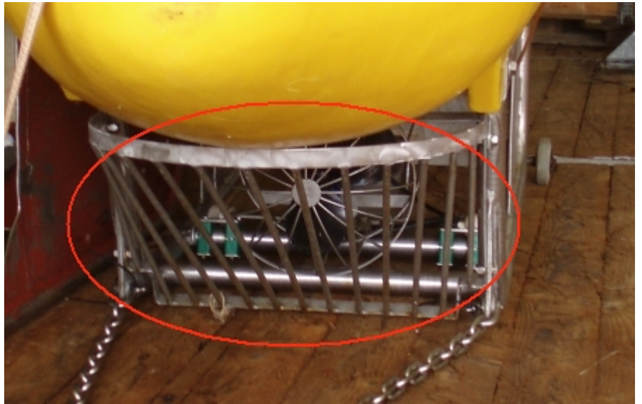
Figure 10. Exclusion 'turtle guard' design (the added structure is circled in red)
