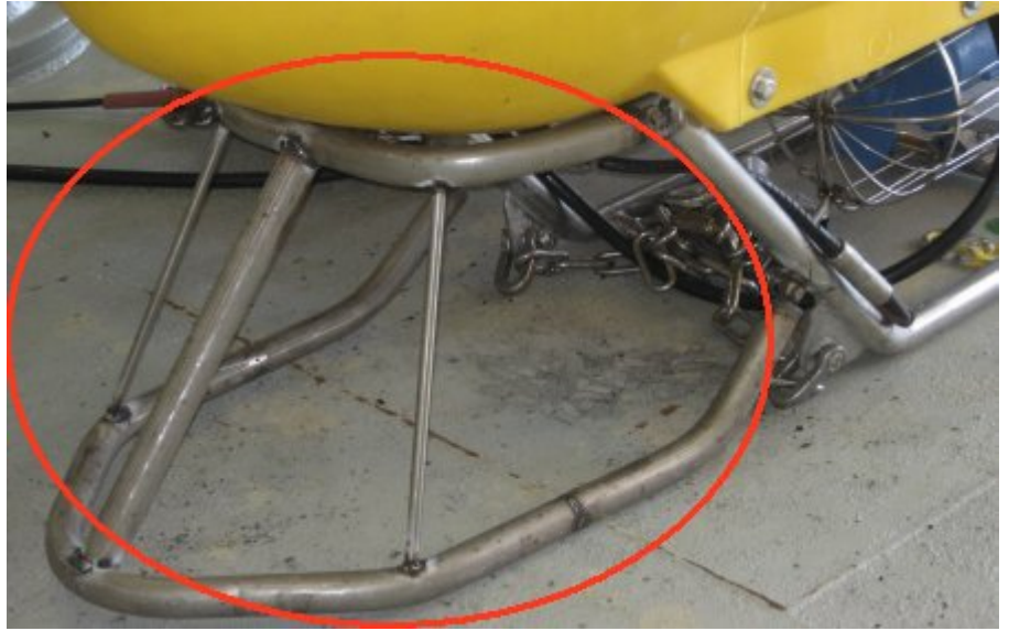
Figure 12. Forward-projecting deflector turtle guard design (the added structure is circled in red)
