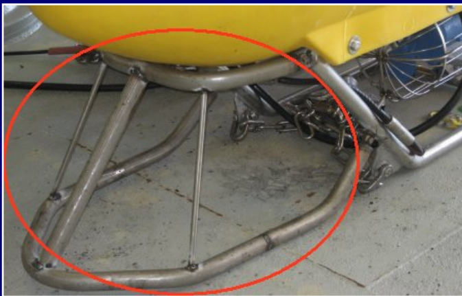
Figure 10. Forward-projecting turtle guard design (the added structure is circled in red)
