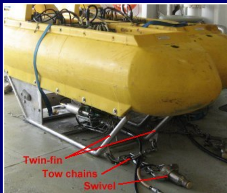
Figure 5. A tail buoy on deck, showing the twin-fin design, swivel and tow chains
