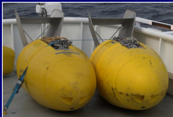
Figure 6. Two dilt floats on deck (upside down) showing the twin-fin subsurface structure
